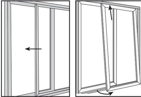
2. Lift up on the panel so the top of the panel pushes fully up into the head of the door frame.
